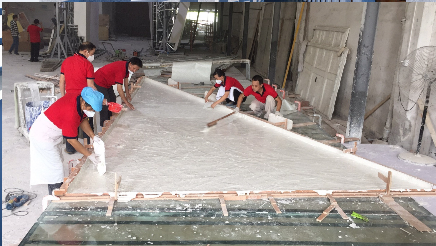
GRP Feature Ceiling System Lamination
